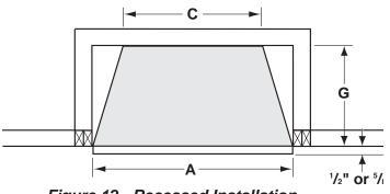
Figure 12 - Recessed Installation
